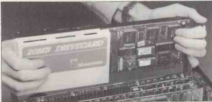
Cards are convenient for upgrading but make heavy demands on the power supply.
