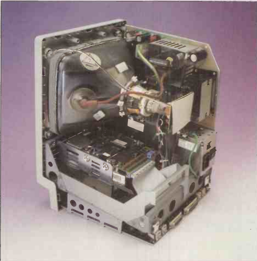
Above: A lot is packed into the limited space inside the SE. Right: The 256Kbit RAMs can be replaced by larger chips to boost the memory.
