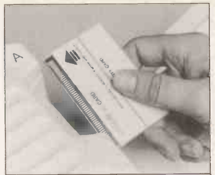
Extra founts are loaded from cartridges not much bigger than credit cards.
